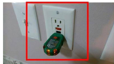
GFI Outlet failed trip test
