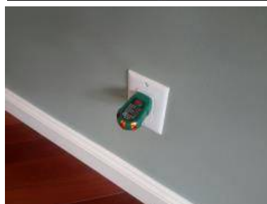
GFI Outlet failed trip test
